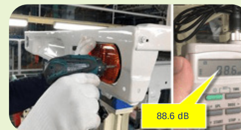
▲ Noise reduced to 88.6 dB after switching to fixed-torque electric screwdrivers
